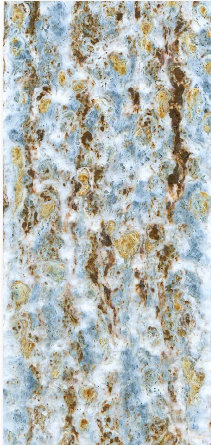
Batch galvanised 83 \mu\text{m} after 12 weeks
